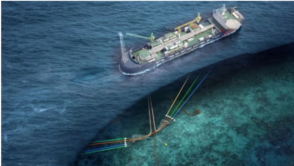
Figure 3-7 Artist's rendering of proposed Bay du Nord FPSO, with subsea manifolds pipeline bundles and riser
