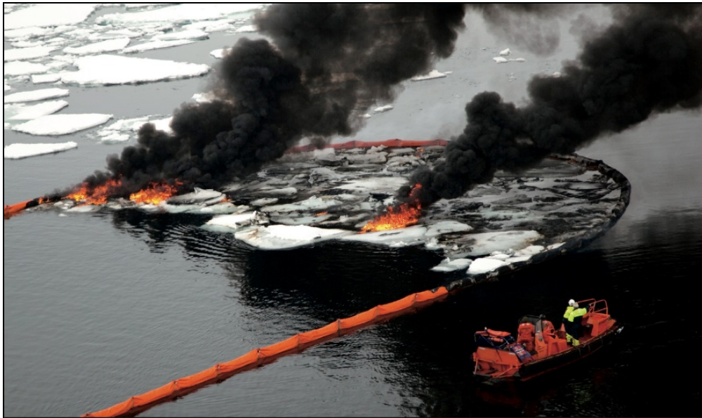
Photo 2-1 Burning crude oil spilled into a field of small ice cakes collected in a fire-resistant boom.
